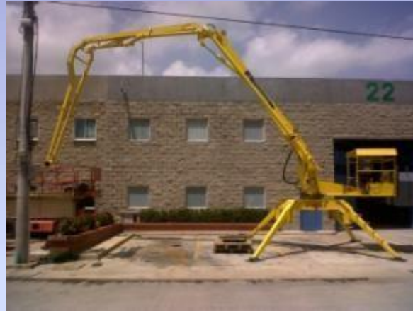
Placing Boom 17 metros
